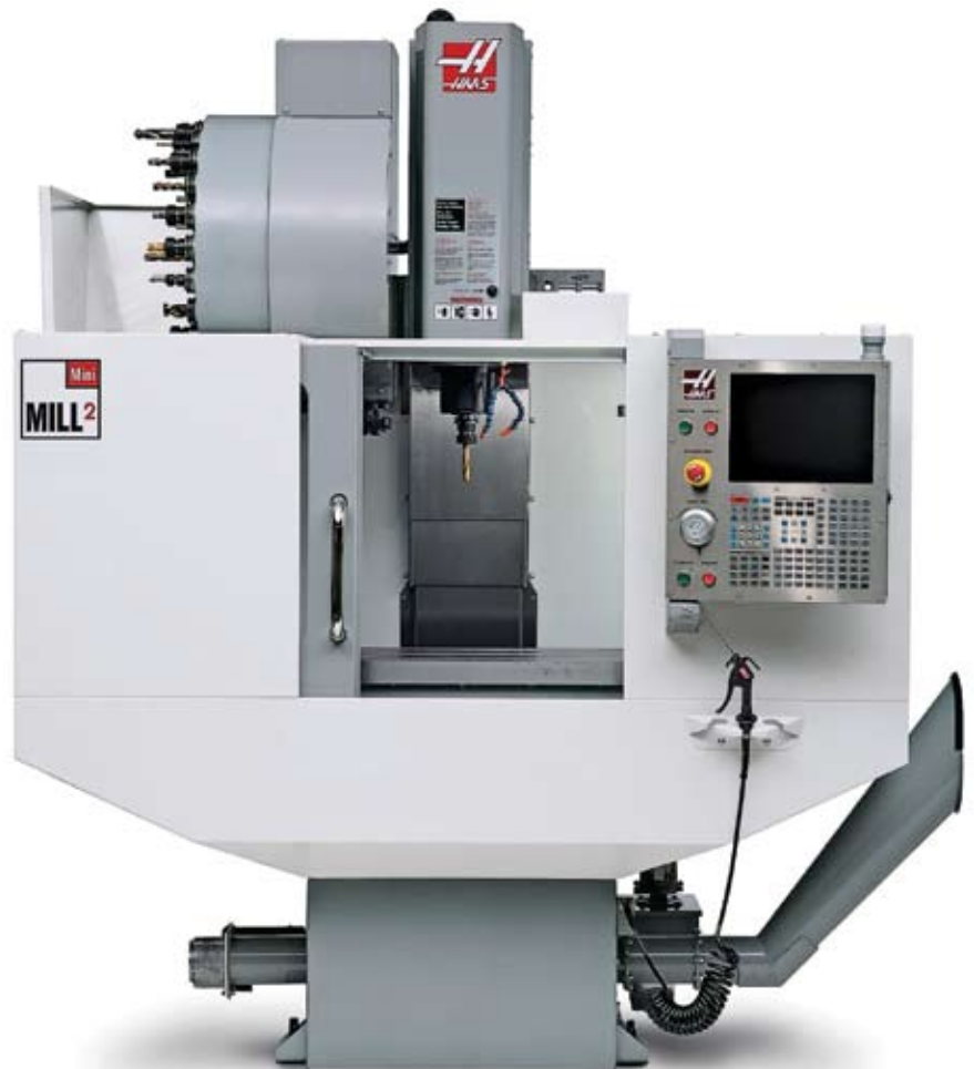
The Haas Mini Mill 2, with extended travels of 508mmx405mmx356mm for the X, Y and Z axes, respectively, has a 40-taper spindle capable of spinning up to 6,000 rpm.
