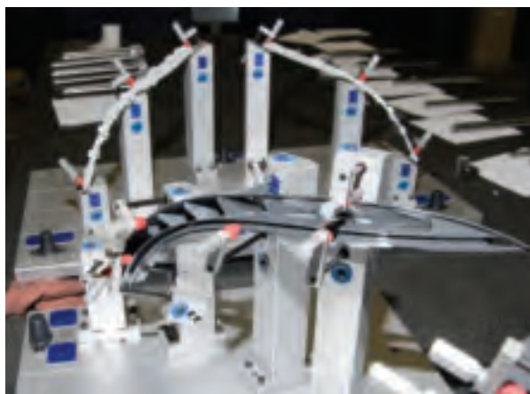
Cavalier specializes in applications with high glass filler content, including fans, shrouds, radiator intakes, door carrier plates, door panels and lighting tools, such as this one for an automotive head lamp.
