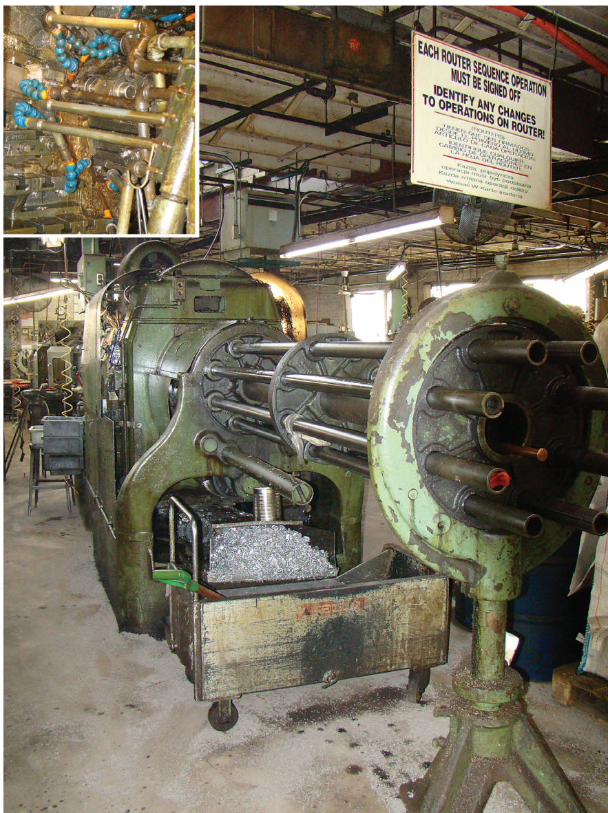
An Index machine custom-built with eight tools in a turret instead of the standard six.
